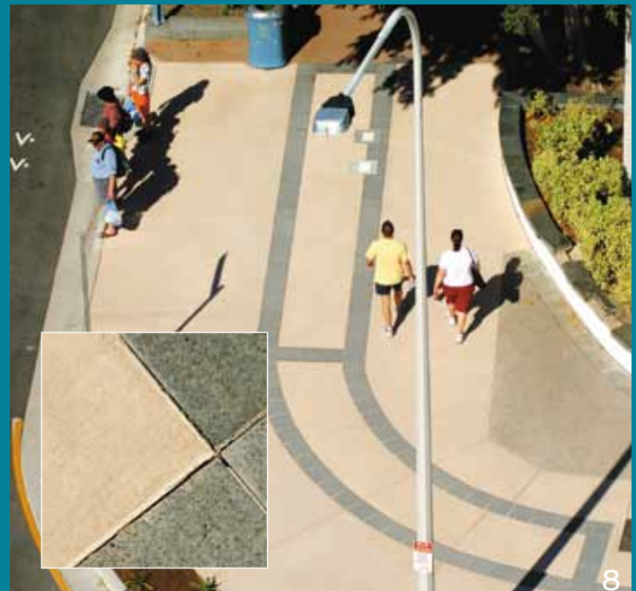
8 Coloured concrete helps define pathways for pedestrians. CCS Driftwood was used in the concrete together with charcoal paver inserts.
