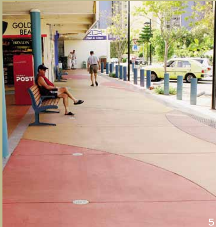
5 Four CCS colours were utilised together with sandstone inlays to create an attractive, yet comfortable footpath setting to the main shopping precinct at this regional centre. Concrete coloured with CCS Cardinal, CCS Biscuit, CCS Chocolate and CCS Honeycomb.
