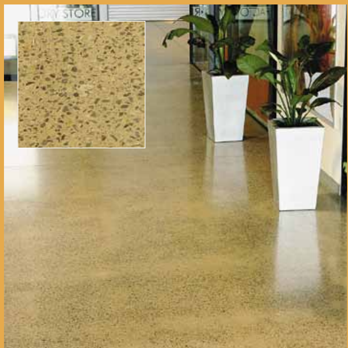
6 The Direct Factory Outlet Centre in Brisbane incorporated polished concrete within the main thoroughfare areas. A distinctive but similar coloured aggregate to CCS Lemon Cream was used to provide the contrast. Architect: S.P.L.A.T. Qld.
