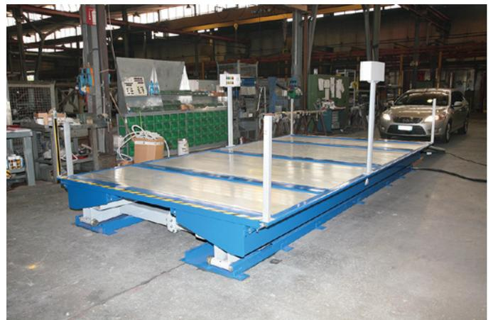
The platform is built with a series of galvanised panels which are both extremely sturdy and also light.
