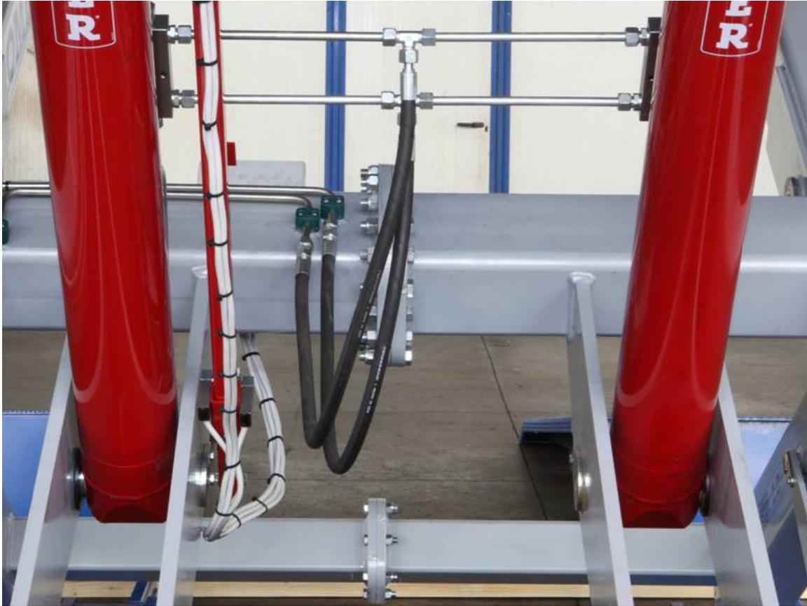
Heavy duty hydraulics allow maximum load lift. Built in valves for reading pressure differential and ensures safety which is a prime consideration.
