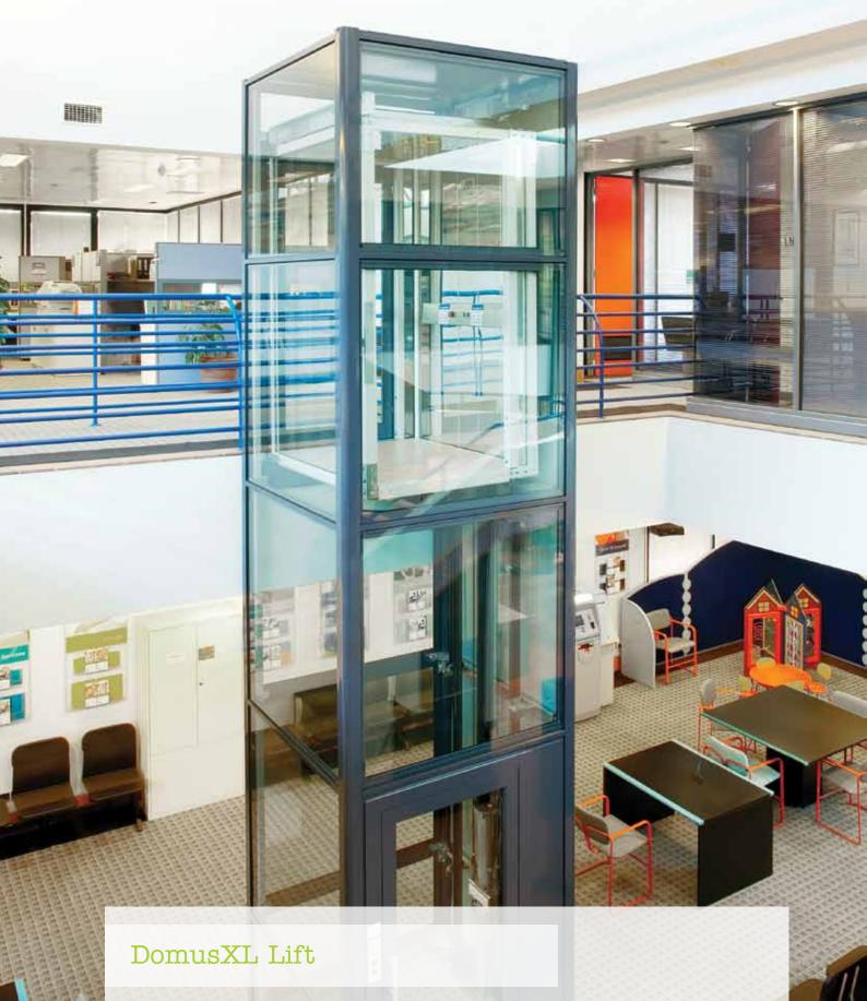
The economical hydraulically operated 1100x1400 DomusXL Lift with swing landing doors is our most popular model in both private residential and commercial (limited mobility) applications. Complying with the BCA and both AS1735.18 & AS1735.15 with a lifting capacity to take 4 adults or a wheelchair occupant and a carer.
