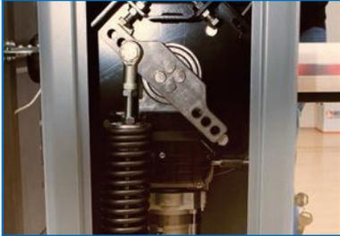
The boom gate cabinet is strong, robust and very stable during operation. 3 mm steel plate zinc coated finished in white polyester UV resistant powder for long life.
