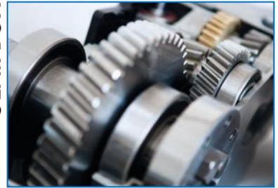
Steel machined gears assembled with high quality bearings are rigorously tested to ensure precision movement and a long life.
