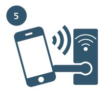
After ensuring that the Bluetooth is enabled, the resident simply holds the smartphone to the door lock, waits for the solid green light and enters the room.
